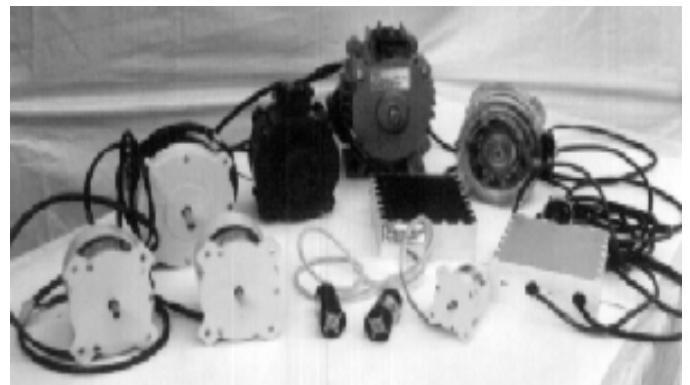
Different type of Motors like BLDC, PMSM, SRM with their Electronics Drives
