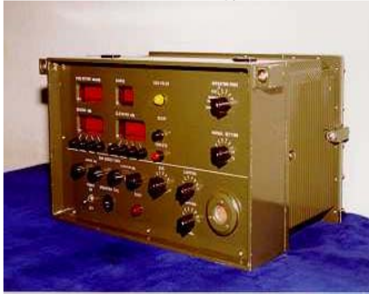
Data Display Unit for 155 mm Field Howitzer Gun for indirect Firing
